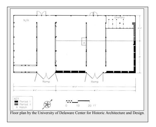
Windom Mill barn floor plan, main block. The plan does not show the rear outshed or the gableend machine shed. This barn originated as a stone barn and was enlarged twice. University of Delaware Center for Historic Architecture and Design.
