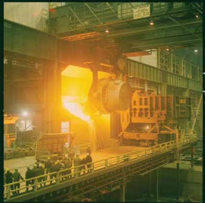
Hot Metal Charge in the Basic Oxygen Furnace, Bethlehem Plant, 1968. From the National Museum of Industrial History permanent collection.
