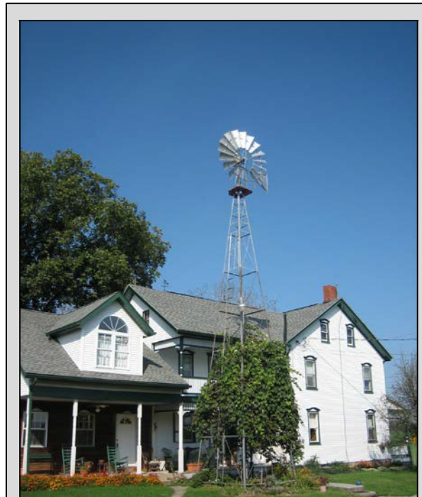
Aermotor USA A-702 windmill, Bethel Township, Lebanon County. This model was manufactured between 1933 and 1969. This particular windmill probably dates between 1933 and 1950. It ran a pump which is still attached, though no longer used. Site 075-BE-001.
