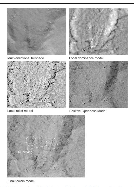
Figure 3. LiDAR derived terrain models. The final terrain model has been used to highlight areas of potential quarrying, which are then field verified. As seen above, quarry pits cover the hillside. Wagon roads and a charcoal hearth are also visible.
