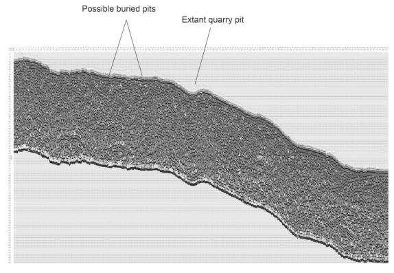
Figure 5. Example of a west to east GPR radargram from 36AD0569. Our interpretation of the data is that there are likely 2 buried quarry pits just west of a large pit that is still apparent on the surface.
